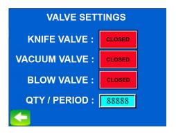
Knife Valve: Manually close knife valve.
